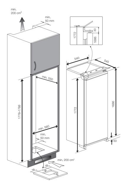
The backwall of the wooden cabinet must be left open completely to kitchen wall in order to allow sufficient air circulation to cool down the condenser unit for energy efficiency.
