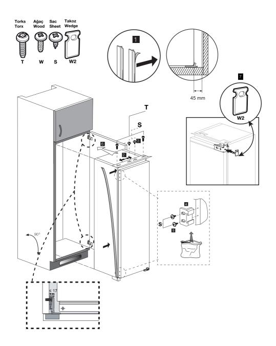
NOTE: When assembling 2, leave the screws loose enough to adjust the part left or right.
