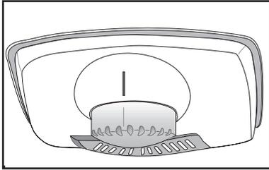
Operating temperatures are controlled by the control (see diagram) located on the ceiling of fridge compartment. Settings may be made from min, 1 ... 6, max, max being the coldest position.
